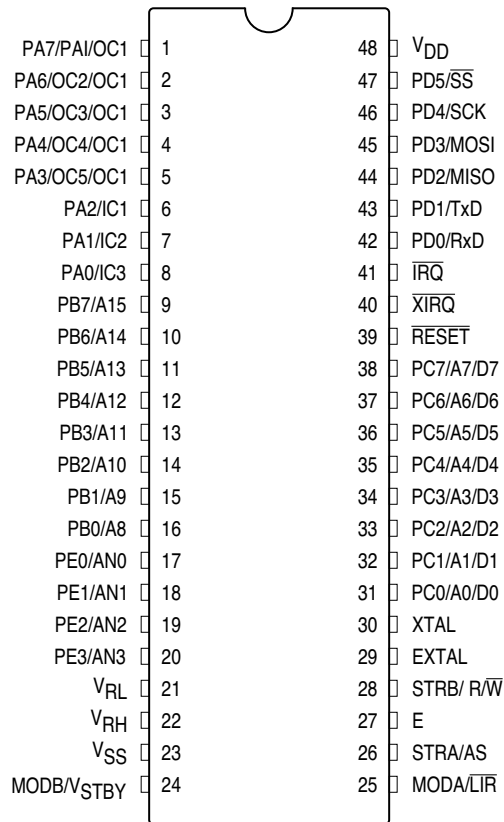
Figure 3 48-Pin DIP Pin Assignments
