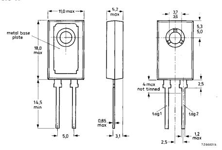
The exposed metal base-plate is directly connected to tag 1.
